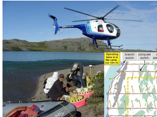
LEFT - Crew prepares for wiring the lake areas with floating electronics (yellow-pink) and GPS positioned lake-bottom electrodes.
